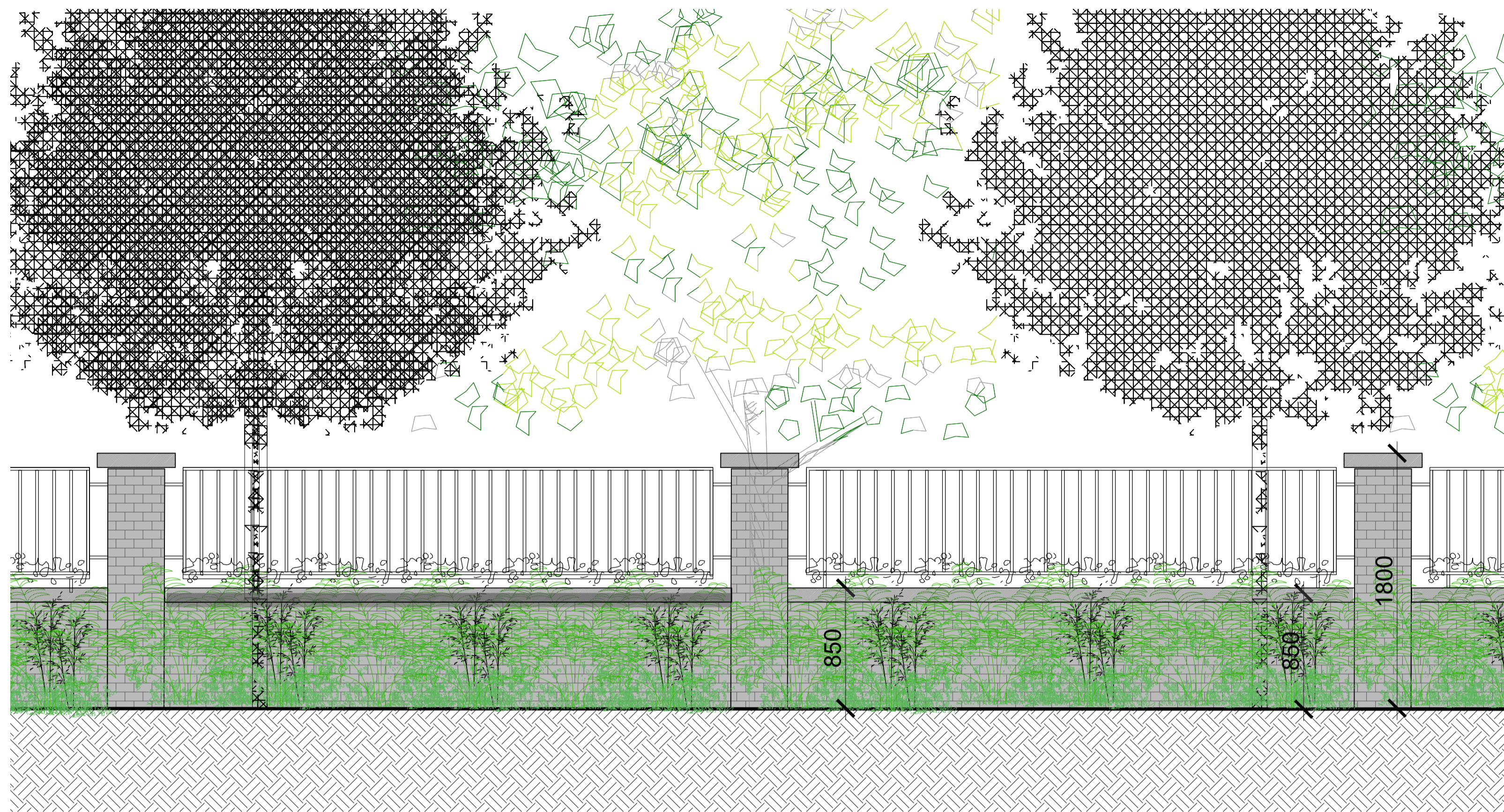
01 TYPE 1 1800mm HIGH BRICKWORK & PAINTED METAL RAILING OVER BOUNDARY TREATMENT TO COMMUNAL AMENITY AREAS FACING AREA AT CAIRNS ROAD FOOTPATH & PUBLIC REALM 1:25 @ A1
